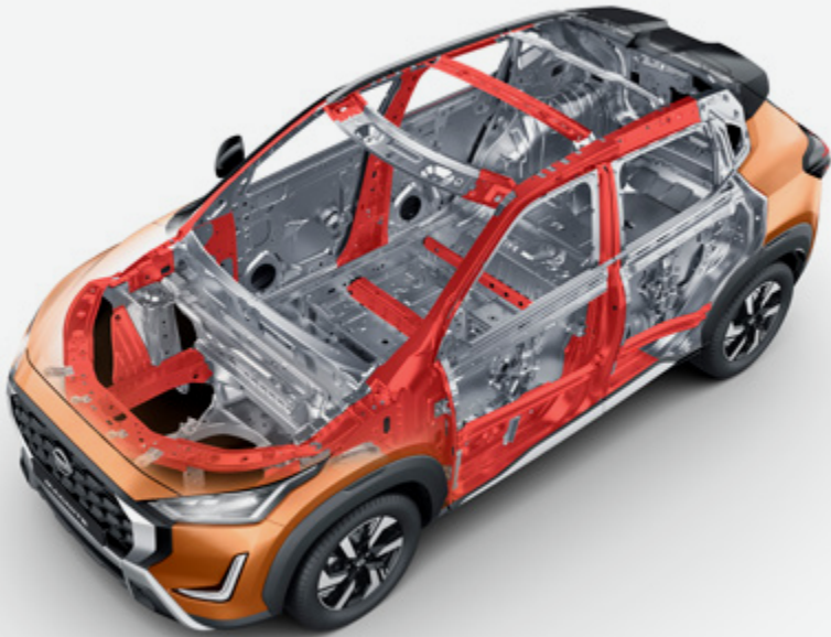
67% Usage Of High Tensile Strength Steel
